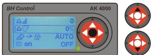
Fan adjustment is possible in case you need to increase or decrease amount of air. This figure is possible to adjust from -5% to +15%. Figure adjustment to „0“ meets pellet quality EN Plus A1.
