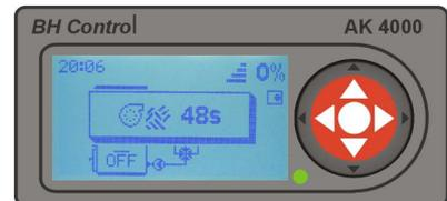
Pressing „ENTER“ display offers round button. Pressing button ◀ boiler will shut down. After shutdown, the blowing fan is switched on. During 60s period pellet burner is being cooled down. By pressing ☒ round button will disappear.
