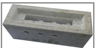
Ceramic nozzle is made of special heatproof concrete designed to mix gases with secondary air to ensure ideal combustion. The nozzle is placed inside previously prepared gap. Area around nozzle is filled with heatproof concrete at the same height as the nozzle. Nozzle lifetime depends on its mechanical wear caused by fuel adding or poking the fire base. Change nozzle if necessary.
