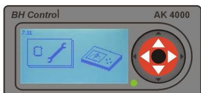
By pressing „ENTER“ service settings can be recalled. Using buttons ▲▼ choose parameter, by pressing „ENTER“ figure starts flashing.
