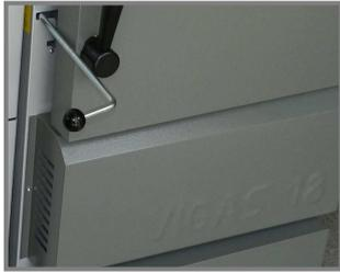
Flap position affects quality of combustion. The correct proportion between primary and secondary air is set by screws „1“. Ideal set up of secondary air is 1,5 turn of screw „1“. If you need to change or check setting, follow these steps:
