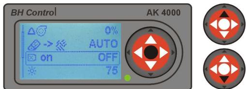
In case of installation and selection of discharge fan (see chap.10.1.3), there is possibility using it to increase chimney effectivity by permanent running. Possibility to adjust speed from 30% up to 100% or completely shutdown to „OFF“.
