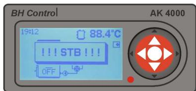
„STB“ failure is caused by boiler overheating. Aktivovala sa tepelná poistka. When this happens, the thermal fuse is activated and fan is disconnected from the power supply (pic. 3/7). Boiler can be only switched on if STB fuse is reset manually (picture), when boiler temperature drops down to **60°C**. To switch on the boiler press „ENTER“ button.
