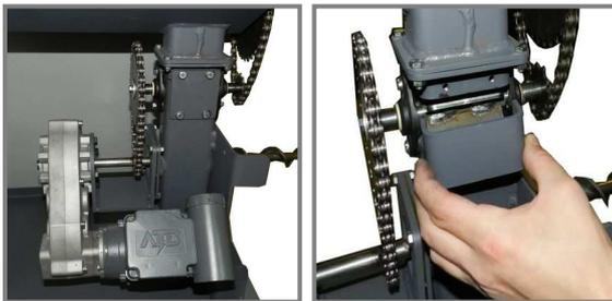
Chamber pellet dispenser (tourniquet) is the device designed to transfer required amount of pellets into the feeder and to create separate air space above feeder. The construction of the driver using chain transmission will avoid pellets to catch fire inside container. This design also provides easy checks and cleaning, if tourniquet is jammed with unwanted object.
