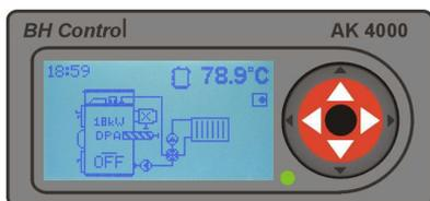
Symbol „OFF“ will appear, as shown on the picture, if boiler is switched off, by pressing middle button „ENTER“, round button pictogram appears.
