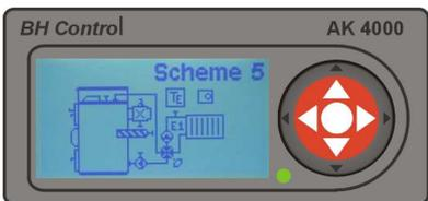
**Schema 5** used with one heating circuit for floor or radiator. Central heating temperature can be controlled according to external temperature, room thermostat or by combination of both. The boiler pump and central heating pump are controlled separately. Boiler protection against low-temperature corrosion provides 4-way valve with servounit.
