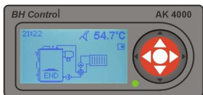
When exhaust gas temperature drops down below desired temperature (end) boiler will shut down with symbol „END“ on the display. If you selected automatic switch from „WOOD“ fuel to „PELLETS“ → , boiler will be switched on – pellet ignition mode and boiler continues running to the desired temperature.
