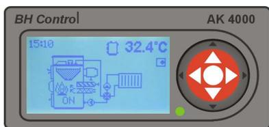
Ignition mode shows symbol „ON“. It is automatic process supported by chimney temperature monitoring.
