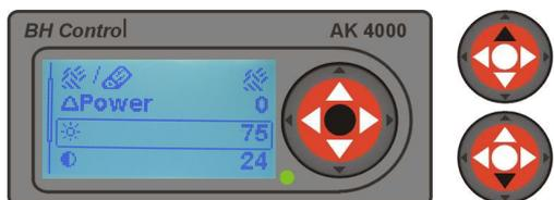
Select figure for display brightness. This figure is possible to adjust from 0 to 100.
